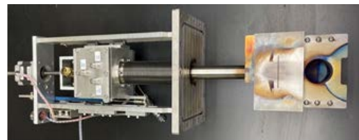
Figure 12. Integrated Faraday cup with an Allison type emittance scanner
