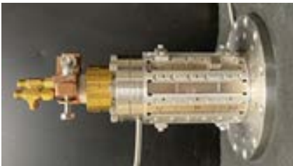
Figure 3. Second smallest 300cc plasma volume H-/D- ion source with off the shelf filament holder.
