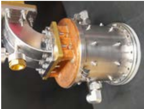
Figure 8. Standard 1200cc H- ion source with its 2.54GHz microwave injection system. This source also can produce any negative ions as well as positive +1 or +2 ions from gaseous or solid elements.
