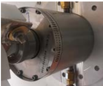
Figure 2. Smallest 125cc plasma volume H-/D- ion source developed at TRIUMF with its screw-in type filament holder.
